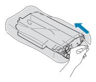
**9** Remove the paper covering on the transfer belt by removing the tape.
